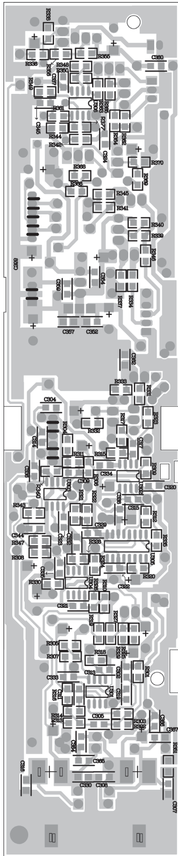
Figure 11. Input/Limiter PCB (Non-RoHS) Top Side Etch Layout
