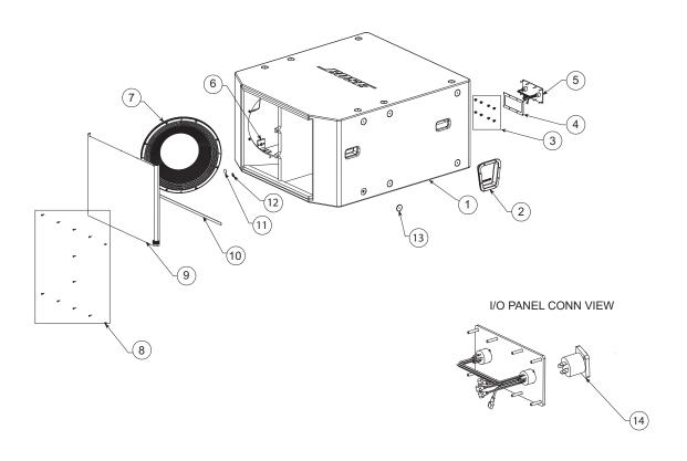
Figure 2. RoomMatch RMS218 Subwoofer Exploded View
