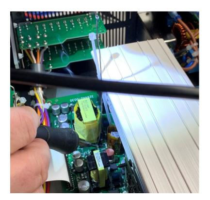
c. Remove the diode using the tweezer iron.
