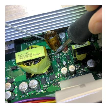
b. Tack the part in place with careful attention to polarity using a single iron and a regular tweezer. Cathode stripe should be towards the Digital board.
