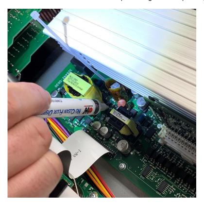
b. Add solder to each end of the diode using a single iron.
