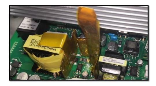
2. 16 AWG Copper wire to hold FCC cable away from the board. Bend its ends and hold it in place on the Digital board as seen below. This will be the FFC cable retainer.
