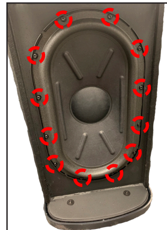
Figure 18. Woofer Screws Removal
