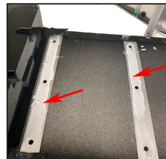
Figure 7. Heat Sink Thermal Grease
