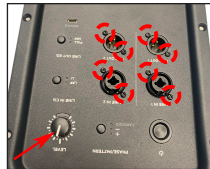
Figure 14. 4 Jacks Screws & Level Knob Removal
