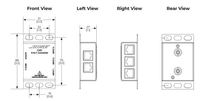
1. Dimensions are shown in millimeters over inches.
