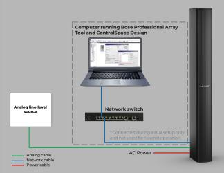
In this configuration, the MSA12X offers a convenient 'set it and forget it' approach by receiving an analog line-level source. Once the beam is aimed and programmed, the computer and network switch plays a role in the initial setup and can subsequently be disconnected, resulting in a cost-effective analog solution.
