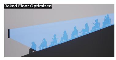
Raked floor optimized is good for covering a raked floor or flat floor from a relatively high array position. Radiates using a vertically asymmetrical beam.
