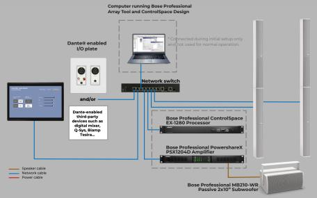
The MSA12X introduces the capability of beam preset recalls, accessible through the ControlSpace Remote app running on a tablet, as depicted on the left. With a simple press, these buttons can activate presets that dynamically adjust the MSA12X's beam.
