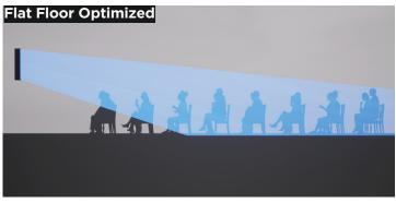
Flat floor optimized is ideal for flat floor seating with the array bottom mounted slightly above ear height of audience. It provides consistent coverage from the front to the back row.
