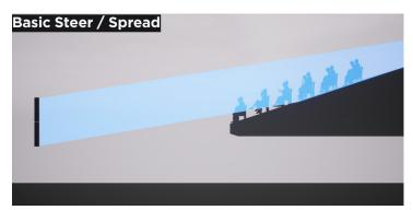
Basic steer / spread is the most basic beam pattern. It allows steering the axis of the beam vertically, then spreading the beam from that axis.
