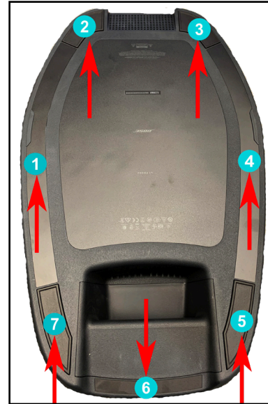
Figure 4. PC Sheets & Rubber Feet Location
