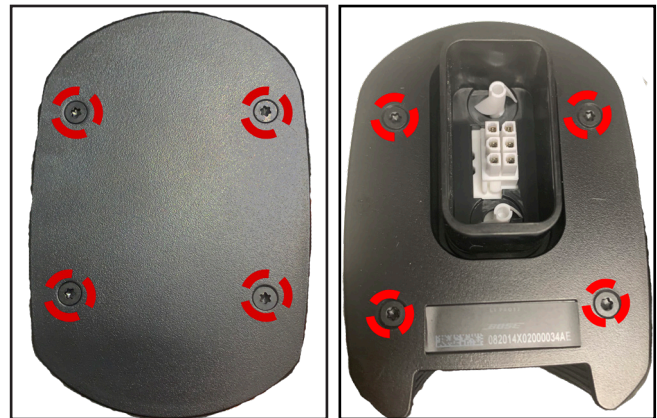
Figure 16. Both Ends of Endcaps Screws Removal
