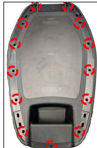
Figure 6. Bottom Cover Screws Removal
