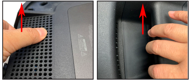
Figure 7. Bottom Cover Removal
