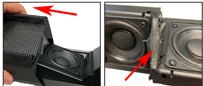
Figure 18. Array Grille Removal & Gasket Material Location
