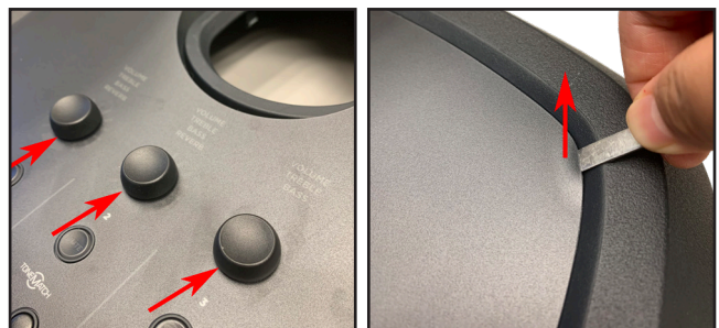
Figure 10. Volume Knobs & Top Cover Removal
