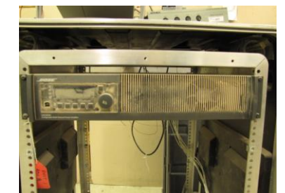
Accelerated dust accumulation – 22 years of dust shown.
