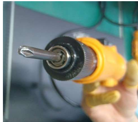
Crosshead bit Spec: PIL-BASD-6600L+ T5*60*40*1
