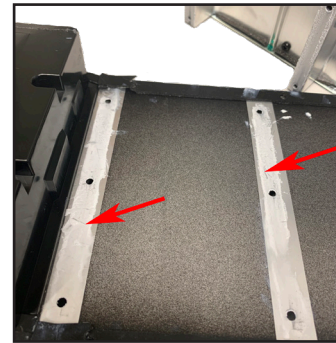
Figure 16. Heat Sink Thermal Grease
