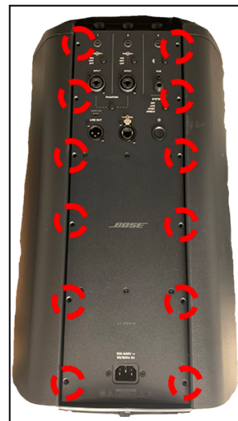
Figure 11. I/O Panel Assy Screws Removal
