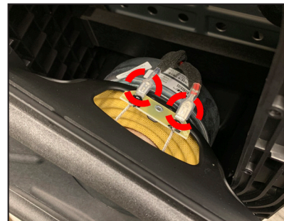
Figure 24. Press the White Fastener
