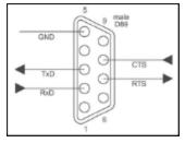
RS-232 Panel Connector Pinout (DTE)
