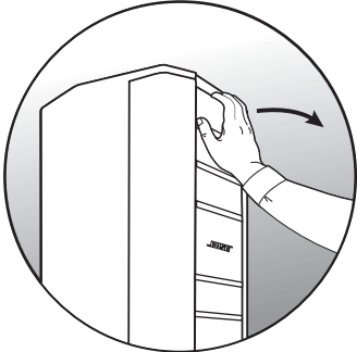
Pulling an array out
