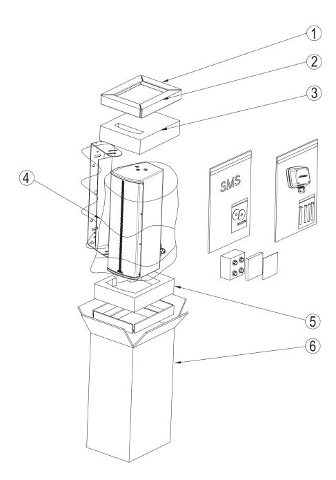
Figure 6. RMU206-WR Top Level Assembly
