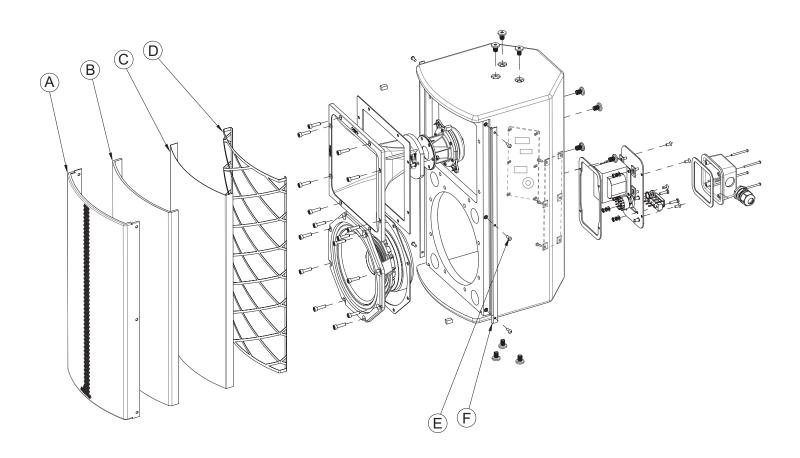
Figure 5. RMU108-WR Main Assembly Exploded View
