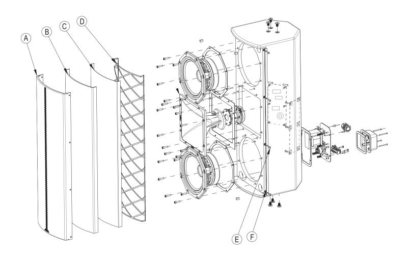
Figure 9. RMU208-WR Main Assembly Exploded View
