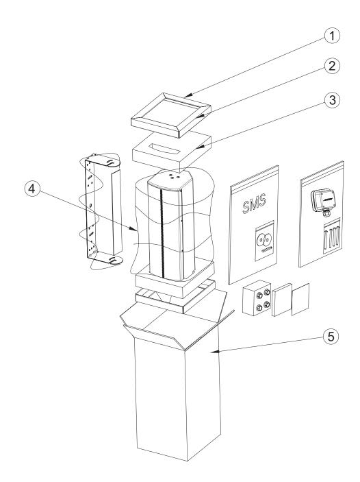
Figure 8. RMU208-WR Top Level Assembly
