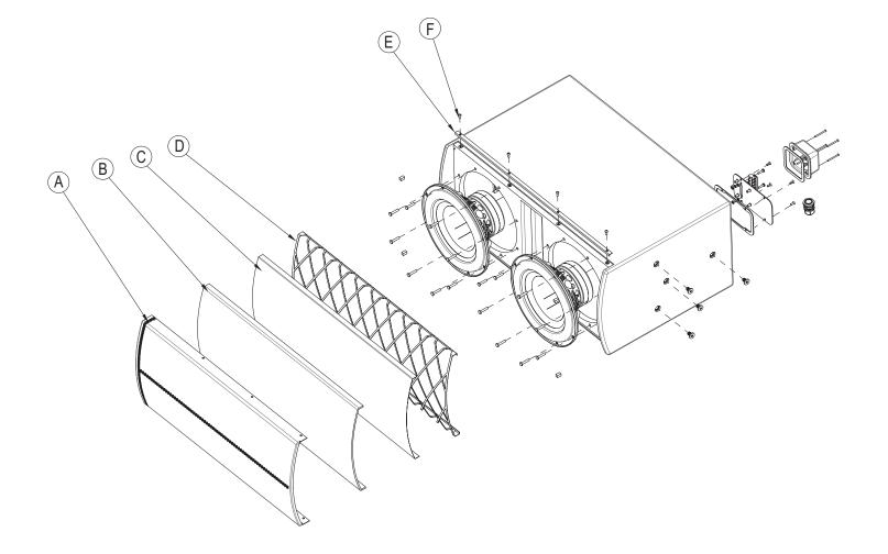
Figure 11. MB210-WR Main Assembly Exploded View
