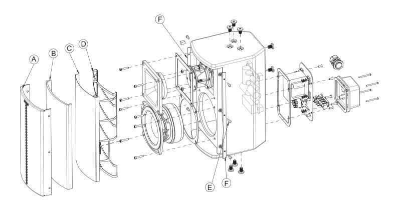
Figure 3. RMU105-WR Main Assembly Exploded View
