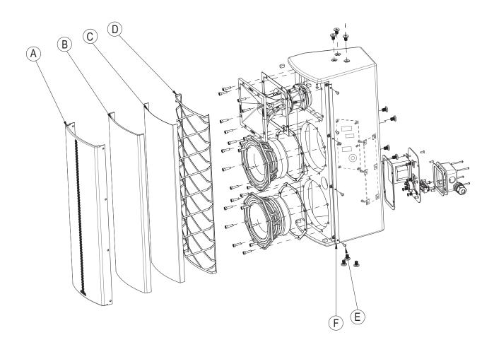
Figure 7. RMU206-WR Main Assembly Exploded View
