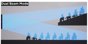
By utilizing all the drivers of the array for both beams simultaneously, Dual-beam mode allows you to use any two beam patterns independently.
