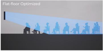
Flat-floor optimized is ideal for flat floor seating with the array bottom slightly above ear height of audience. It provides consistent coverage from the front to the back row.
