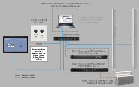
The MSA12X introduces the capability of beam preset recalls, accessible through the ControlSpace Remote app running on a tablet. With a simple press, these buttons can activate presets that dynamically adjust the MSA12X's beam.
