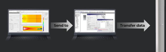
**Bose Professional Array Tool** is the first step in designing the MSA12X into the room. It is a simulation and analysis software that allows audio system designers to define venue parameters, position the MSA12X, and accurately predict its performance.
