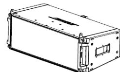
**ShowMatch SM20 full-range module** with 20° vertical coverage. Ships with 100° horizontal waveguide installed and includes 70° waveguide panels. Change single panel for asymmetrical coverage. Optional accessory: 120° horizontal waveguide.
