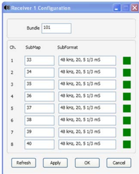
Configuration Panel showing new Bundle assignment and on-line status
