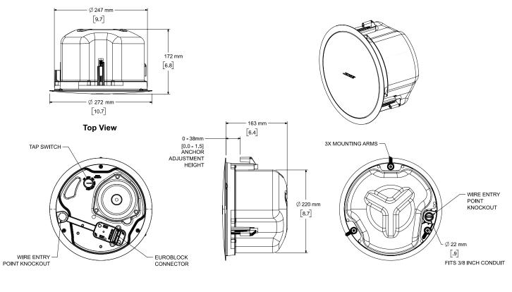
Front View GRILLE AND CAP REMOVED FOR CLARITY Right View DIMENSIONS APPLY TO BOTH SIDES
