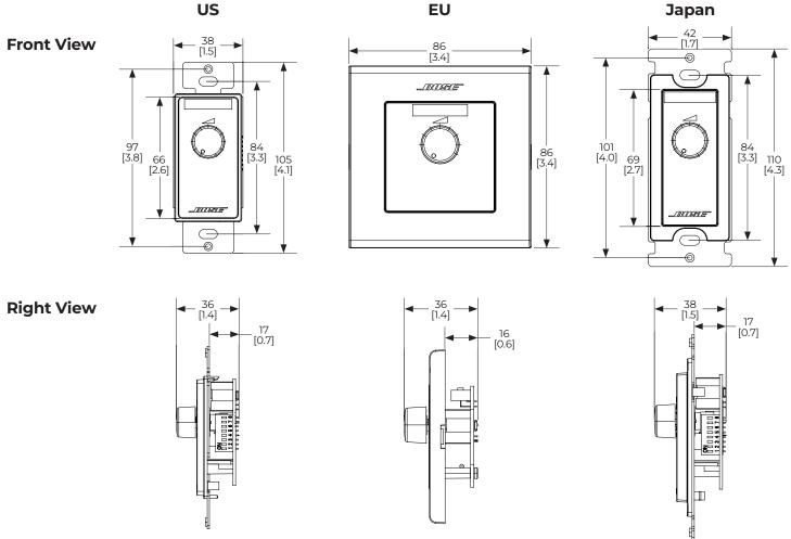
2. Dimensions are shown in millimeters over inches.
