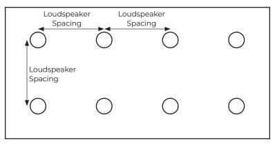
D. After the last loudspeaker is placed, center the loudspeakers in that row to create new offset distances out from each wall, which may be unique from  $\frac{1}{2}$  LSD.
