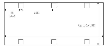
C. After the last loudspeaker is placed, center the loudspeakers in that row to create new offset distances out from each corner, which may be unique from  $\frac{1}{2}$  LSD.
